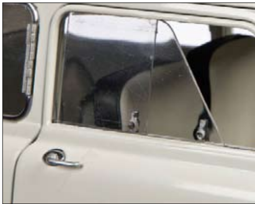
above Monty awards top marks for the sliding door windows – with the correct single-hole catches too.
