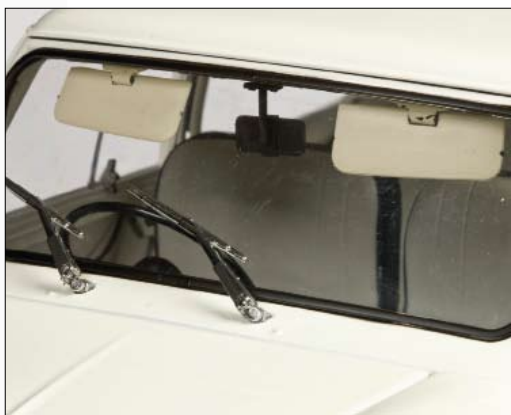
above Front and rear screen rubbers are all black, typical of registration 621 AOK's specification.
